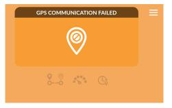
Check the wiring and the GPS antenna for damage and contact Sensor Maritime.
